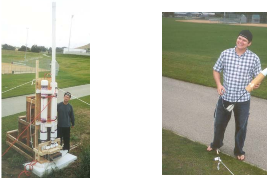
Fig. 36 & 17 Compressed Air Launch Mechanism and Prototype Test Projectile.
