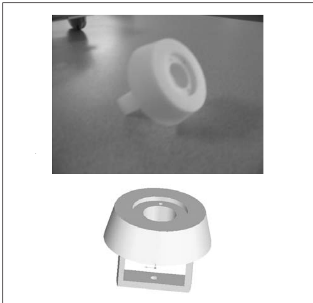
Figure 12 Detail of Camera Fixture in NoseCone
