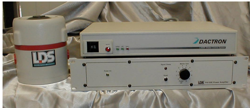
Figure 10. Dactron Shaker Controller, LDS V400 and amplifier used to replicate vibrations.
