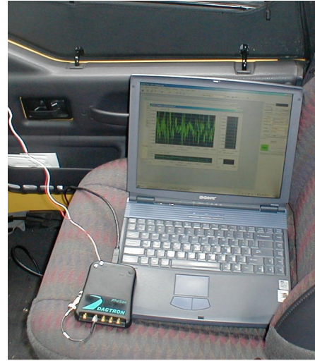
Figure 3. Portable DSA streamed data to disk and displayed real-time spectral and time data to ensure the recorded signals met the needs of the study.
