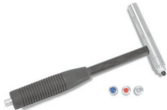
Figure 17. Impact hammer instrumented with a load cell to measure the excitation force and different hardness tips.
